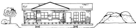
Figure 2. 2000 sq. ft. house prepared for elevation. Approximately 6,500 cu. ft. of dirt will be excavated when all the dirt is removed from beneath the structure. Dirt to be re-used must be kept dry (cover with plastic sheeting). There will be a large hole under the structure until the elevation is complete and fill-dirt has been added. The contractor should be prepared to pump water out of the excavated area in the event of rain.
